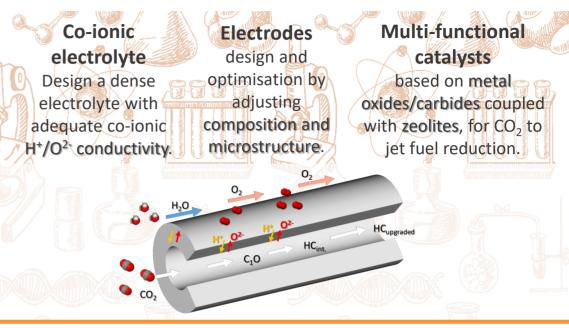
Multi-tube membrane reactor: design, modelling & validation Bench-testing targets a 500 W multi-tubular system, under operating conditions (T = 350-450°C and P > 25 bar).
